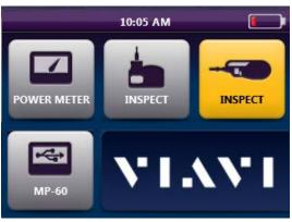
Fig. 4: OLP-82P Home Screen shown with P5000i Probe and MP-series USB OPM attached via USB
