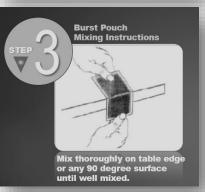
**Step 3:** Use a table edge to mix the resin and hardener (Part A and Part B) or a roller. We recommend counting 25 passes on the table edge to achieve a uniform color and mix. Counting the number of passes (instead of seconds or minutes) helps to ensure a uniform mixture. In each pass, methodically push all the material to one end of the package, then to the other end. Even if the seal is not burst open all the way, it will be burst enough for the material to free flow through the opening.
