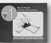
**Step 1:** Roll one end of the pouch toward the burst seal/sealed center dividing Part A and Part B. Roll the side that has the most material in it.
