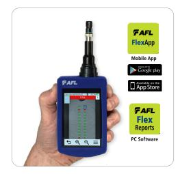
FOCIS Lightning2 focuses, captures, analyzes all fibers in the MPO/MPT end-face with a click of a button!
