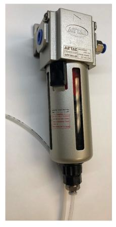
Replacement Filter Elements are Domaille Part# **PM22399**. Install the new Filter Element and lightly tighten with the wrench. Reinstall the Filter Bowl at 45° and turn to engage the latch. Reconnect the air supply.
