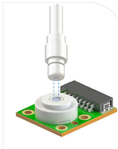
Figure 11. Aperture with 3-mm Lightguide
