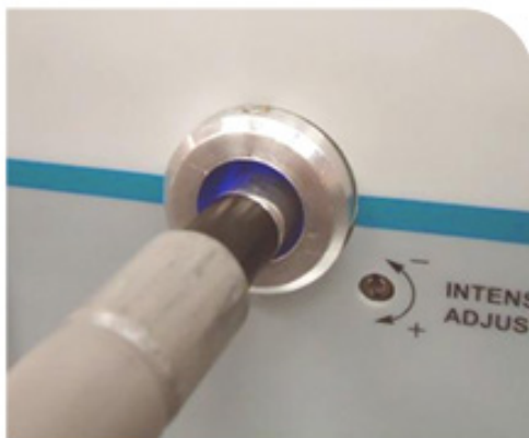
Figure 6. Insert Lightguide into Lightguide Mount
