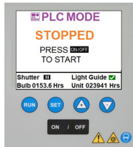
Figure 38. PLC Emergency Stop Function
