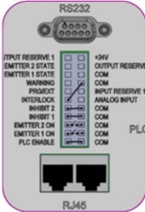
**Note:** The Input/Output terminal block is included in the packaging, with the jumper wires inserted. When the terminal block is installed, the controller will enter PLC mode. PLC mode disables commands and parameter setting from the HMI. To set parameters from the HMI, the terminal block must be removed, or the connection between the PLC Enable and COM pins (1 and 2) must be disconnected.
