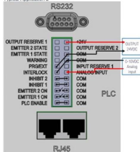
*Note: The Input/Output terminal block is included in the packaging, with the jumper wires inserted. When the terminal block is installed, the controller will enter PLC mode. PLC mode disables commands and parameter settings from the HMI. To set parameters from the HMI, the terminal block must be removed, or the connection between the PLC Enable and COM pins (1 and 2) must be disconnected.*
