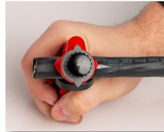
The CST-1140 Round Cable Strip & Ring Tool is designed for fast and precise removal of cable jackets from round cables that are 3/16" to 1 1/8" (4.5 mm-29 mm) in diameter. This round cable stripper features the following:
