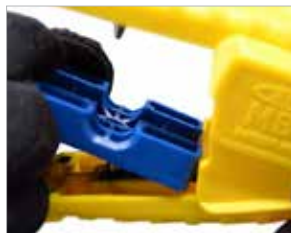
Magnetic trays accurately determine the appropriate blade depth & cable diameter to prevent damage.
