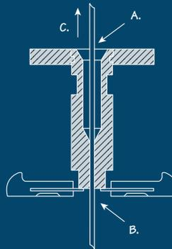
End of fiber guide supports blades during stripping to prevent blade flexing and fatigue.
