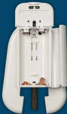
The AA Battery-powered unit has all the same heating, blade and stripping features found on the standard Soft-Strip® tool.
