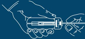
3. With handles closed, pull fiber/wire or cable from tool. Always a precision strip length. Fiber/wire is never nicked or damaged.
