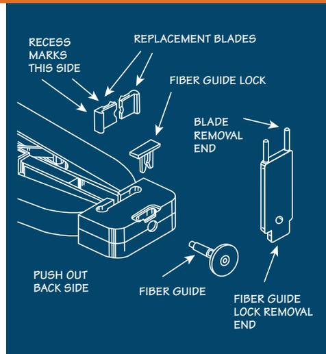
**Note:** *Blades are color coded and matched to diameter and color of fiber guide lock. Replace or install fiber guide and fiber guide lock as needed. Always test strip fiber after installing new blade set. Remove blades periodically and clean with brush provided and alcohol.*
