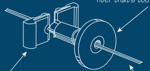
**B.** As gripping handles close, each blade half moves in a straight line to self-align around the fiber guide. This places the blades in perfect concentric relationship.
