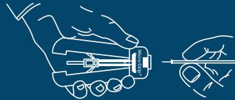
2. Close handles. Blade sets cut almost through the insulation without ever touching the fiber/wire.
