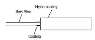
If residual coating remains on the fiber, adhesion between the ferrule and the fiber may be degraded, leading to deterioration of the connector performance. Coating at the root of the bare fiber may be left because it is difficult to remove.
