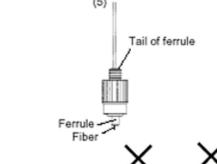
Step 5 Slide the plug onto the fiber slowly. Wipe off the excessive adhesive coming out of the tail of the ferrule.
