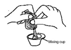
Step 1 Mix the main and curing agents of the adhesive Epo-Tek 353ND according to the instructions printed on the package of Epo-Tek.
