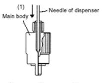
Step 1 Insert the needle of the dispenser into the main body of the plug from the tail until the dispenser stops.
