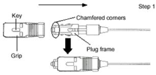
Step 1 Slide the grip onto the plug frame with the key on the grip and the chamfered side of the plug frame facing in the same direction until the grip clicks into place.
