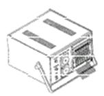
Step 1 Harden the Epo-Tek 353ND by setting the ferrule (with the fiber inserted) into the curing machine OFK-1 or OFK-3. A maximum of 20 ferrules can be cured at a time in the OFK-1 and 24 in the OFK-3 (For more details, see the curing machine manual).
