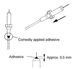
Step 3 Apply a small amount of adhesive on the root of the bare fiber protruding from the ferrule tip to cover about 0.5 mm.
