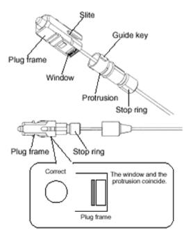
Step 2 Squeeze the stop ring into the plug frame while guide key of the stop ring toward the slite of the plug frame, until the stop ring clicks into place.
