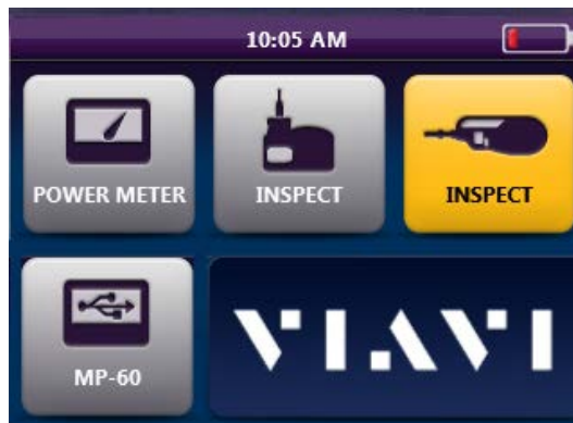
Fig. 4: OLP-82P Home Screen shown with P5000i Probe and MP-series USB OPM attached via USB
